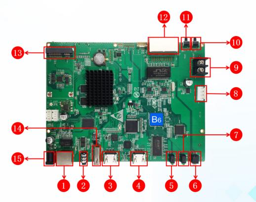
1. Input network port, connected to the computer network port.
