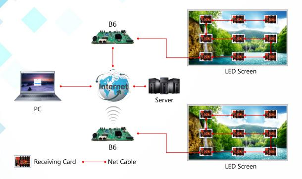
2. Asynchronous one-to-one control: Update programs by network cable connections, Wi-Fi connections or USB flash drives. LAN (cluster) control can access the LAN network through by network cable connection or Wi-Fi Bridge.
